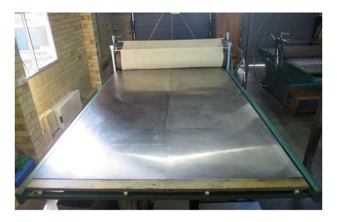
Figure 15 Large-format roller-style etching press, detail of 2m wide bed
