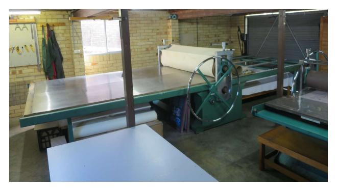
Figure 14 Large-format roller-style etching press
