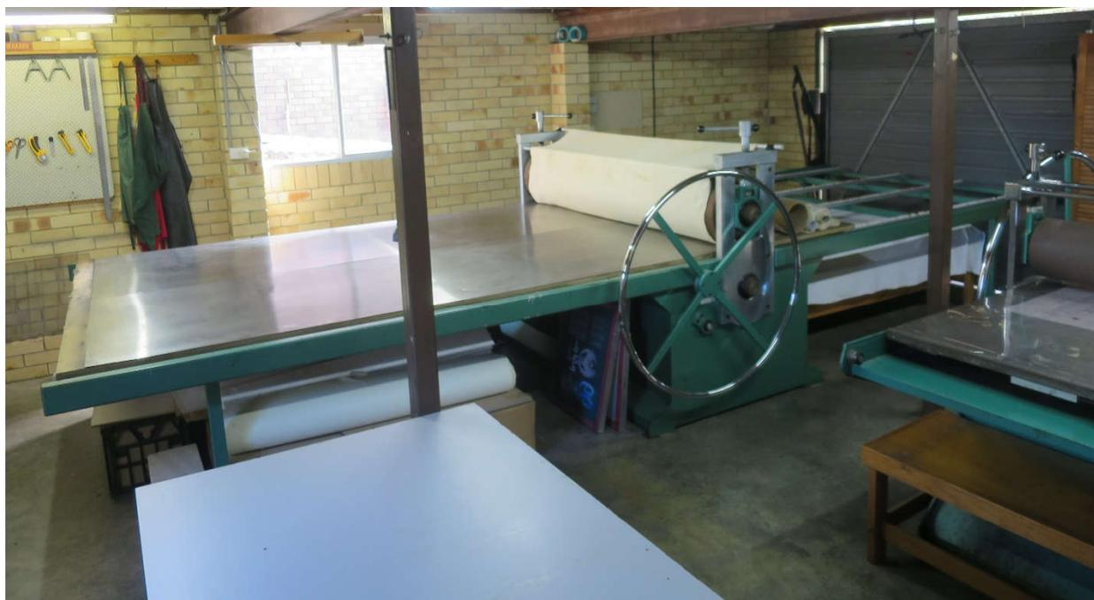
**Figure 14** Large-format roller-style etching press
